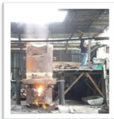
**Gambar 2.** *Melting Chamber*
